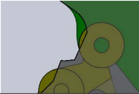
Figure 12: Unnecessary Face Plate Material
