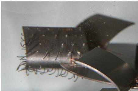
FIGURE 9: Telldaes on BT-6 impeller blade.
