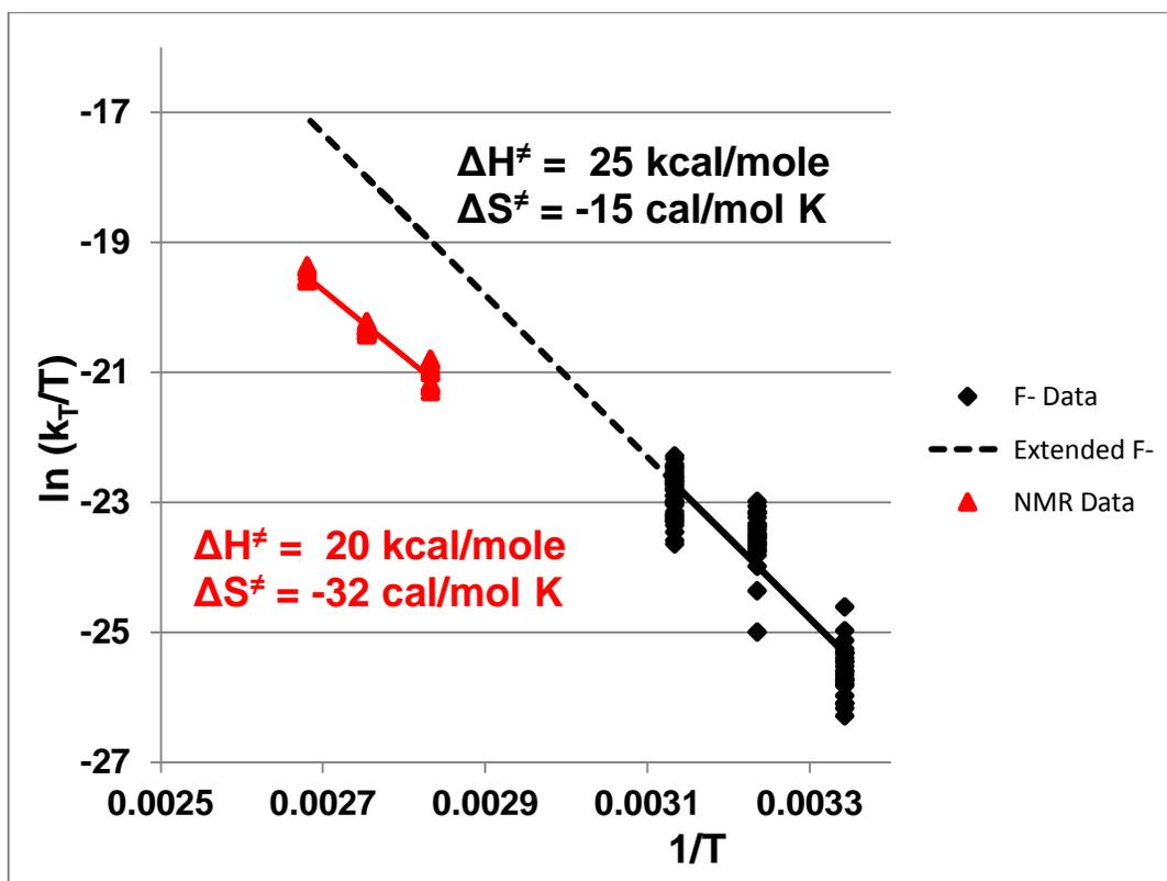
**Figure 5.** Plot of  $\ln(k_T/T)$  versus  $1/T$ , which reveals the experimentally determined activation enthalpies ( $\Delta H^\ddagger$ ) and entropies ( $\Delta S^\ddagger$ ).
