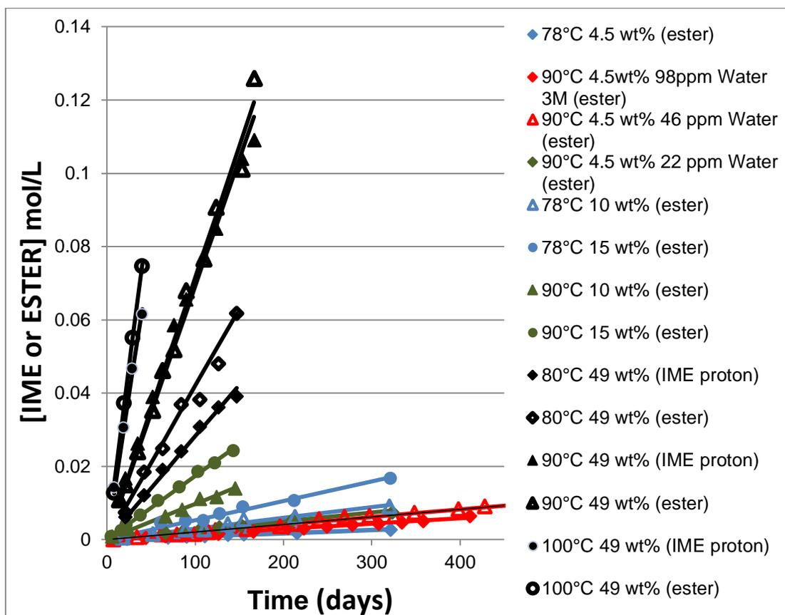
**Figure 4.** Concentration data based on  $^{19}\text{F}$  and  $^1\text{H}$  NMR signal intensities from Novec™-7100/IPA mixtures aged at 78 °, 80 °, 90 ° or 100 °C, with 4.5, 10, 15 or 49 wt% IPA.  $[\text{IME}] = [\text{Ester}] = [\text{Fluoride}/2]$
