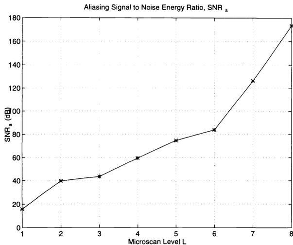
Fig. 5 Aliasing signal-to-noise energy ratio as a function of microscan level.
