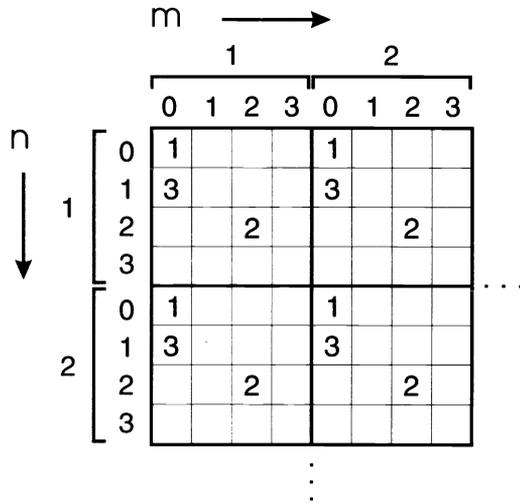
**Fig. 6** Illustration of  $4 \times 4$  high-resolution reconstruction. Image 1 is placed in bin (0,0). Image 2, with a shift of  $(\frac{1}{2}, \frac{1}{2})$  of a pixel, is placed in bin (2,2). Image 3, with a shift of  $(0, \frac{1}{4})$ , is placed in (0,1).
