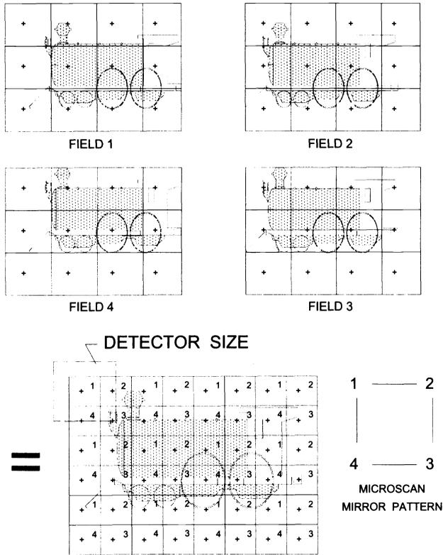
Fig. 3 Illustration of a level-2 microscanning process. The individual images are shifted by half pixels for four separate positions. The reconstructed image has four times as many unique samples as any of the four fields.
