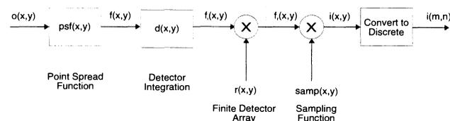
Fig. 1 Basic block diagram of the imaging system.
