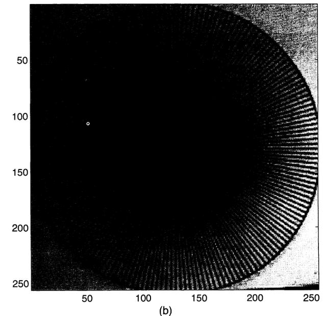
**Fig. 7** Spoke-target comparison. Image (a) is a staring image, and image (b) is a level-2 microscan of the same target. Pixel replication has been applied to the staring image to facilitate a comparison.
