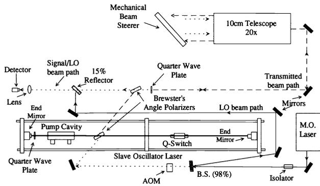
Fig. 1 Experimental setup of the 2.09- $\mu\text{m}$  ladar system.
