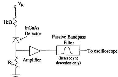
Fig. 3 Detection scheme used with the 2.09- $\mu\text{m}$  ladar system. When this detection package is used for incoherent detection the amplifier is a 60-dB amplifier,  $R_L$  is 16 M $\Omega$ , and there is no bandpass filter. When used for coherent detection the amplifier is a 47-dB amplifier,  $R_L$  is 450  $\Omega$ , and the bandpass filter is 41 MHz.
