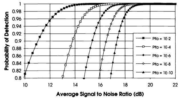
**Fig. 7** Probability of detection plotted against SNR for a glint target using incoherent detection. These curves were calculated using threshold currents of 194.7, 311.2, 397.8, 469.7, and 532.4 nA.
