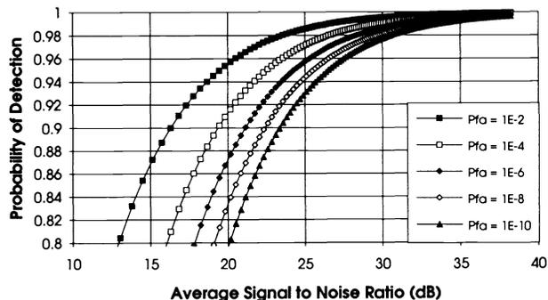
**Fig. 5** Probability of detection plotted against SNR for a speckle target using coherent detection. These curves were calculated using threshold currents for decreasing probability of false alarm of 371.7, 525.7, 643.9, 743.5, and 831.3 nA.
