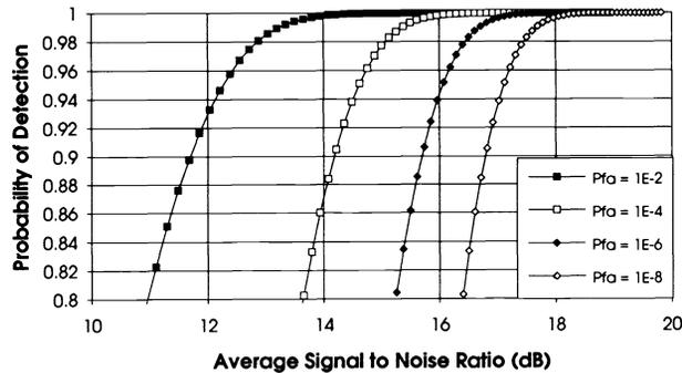
**Fig. 6** Probability of detection plotted against SNR for a glint target using coherent detection. The threshold currents used for each curve for decreasing probability of false alarm are 371.7, 525.7, 643.9, 743.5, and 831.3 nA.
