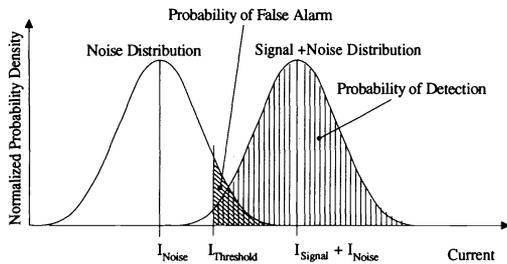
**Fig. 4** Probability of false alarm and the probability of detection for a given threshold current level. The noise distribution is centered at the average noise current and the signal plus noise distribution is centered at the average signal plus noise current.
