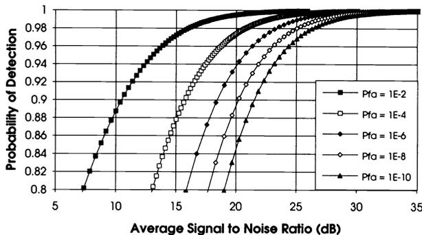
**Fig. 8** Probability of detection plotted against SNR for a speckle target using incoherent detection. These curves were calculated using threshold currents of 194.7, 311.2, 397.8, 469.7, and 532.4 nA.
