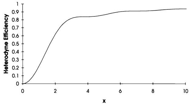
Fig. 2 Heterodyne efficiency for matched signal and LO Airy functions incident on the detector. The expression for the heterodyne efficiency used to plot this curve is  $\gamma = 1 - J_0^2(x) - J_1^2(x)$ .
