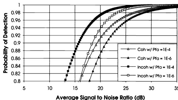
**Fig. 10** Comparison of probability of detection for coherent versus incoherent detection with a speckle target. This plot is a combination of Figs. 5 and 8.
