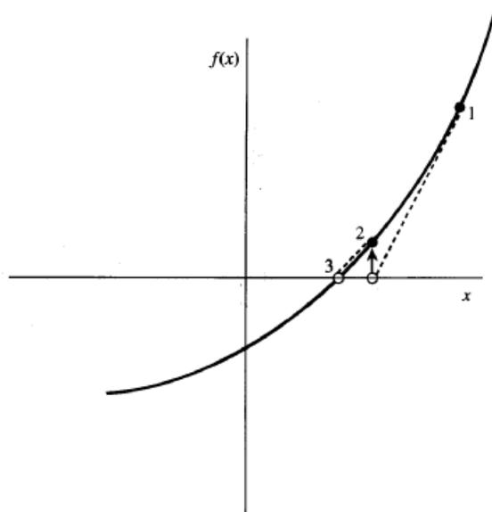
This is an elegant and simple way to determine the roots of a function. However, the Newton-Raphson algorithm can fail in some cases. Two cases where this occurs are shown in Figure 5. If the algorithm encounters a local minimum or maximum the function will evaluate to infinity and never find a root. Similarly, if the function is malformed the algorithm could put itself into an infinite loop, evaluating points over and over again.
