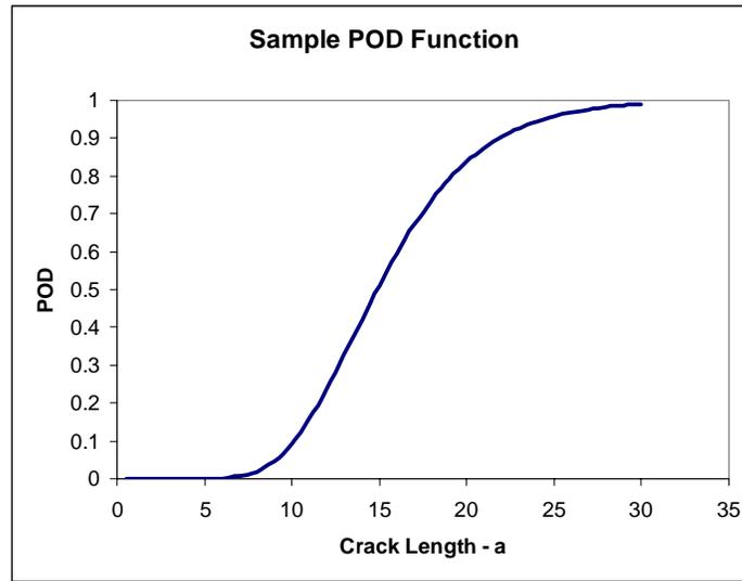
The data that was used to fit to the probability of detection curve came from Pass/Fail inspection results. In the Pass/Fail analysis a set of specimens with known crack sizes is inspected and the inspection result is whether or not the crack was detected.
