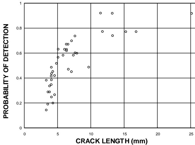
Figure 3 is a depiction of the probability of detection function using the lognormal distribution function shown in equation 1. The parameter  $\mu$  is the logarithm of the crack length that will be detected 50 percent of the time and the parameter  $\sigma$  is a measure of how steeply the central portion of the curve rises.
