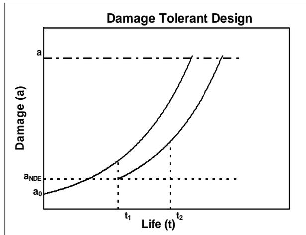
The crack size grows until it reaches size  $a$ , at which the structure fails. In this graph non-destructive inspections are done at times  $t_1$  and  $t_2$ . These inspections are done at half the time it would take the crack to grow to failure. When an inspection is done it reduces
