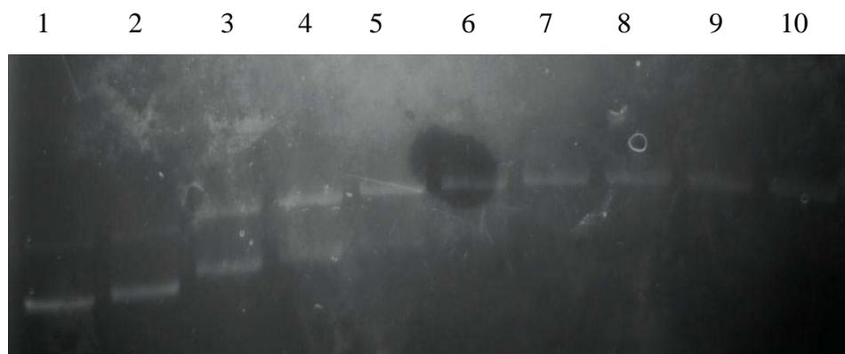
**Figure 5.** Gel electrophoresis of circular plasmid DNA (pUC18) in the presence of complex I (lanes 2-10) and without complex I (lane 1) irradiated with a 300 W mercury arc lamp filtered to allow only light of 420 nm and higher to penetrate, samples taken at 10 min intervals.
