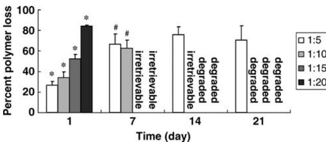
**FIG. 3.** Percent polymer loss of 1 mm diameter hydrogel beads as a function of the crosslinking ratio (1:5, 1:10, 1:15, 1:20). Error bars represent means  $\pm$  standard deviation for  $n = 5$ . \* indicates a significant difference in percent polymer loss compared to the other groups at the same time point based on pairwise comparisons. # indicates a significant difference in percent polymer loss compared to the previous time point in a group.
