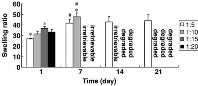
**FIG. 2.** Swelling ratio of 1 mm diameter hydrogel beads as a function of the crosslinking ratio (1:5, 1:10, 1:15, 1:20). Error bars represent means  $\pm$  standard deviation for  $n = 5$ . \* indicates a significant difference in swelling ratio compared to the other groups at the same time point based on pairwise comparisons. # indicates a significant difference in swelling ratio compared to the previous time point in a group.
