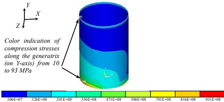
Fig. 9. Stresses in a shell (along the generatrix) (in Pa)
