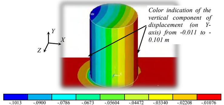
Fig. 5. Vertical displacements (in m)
