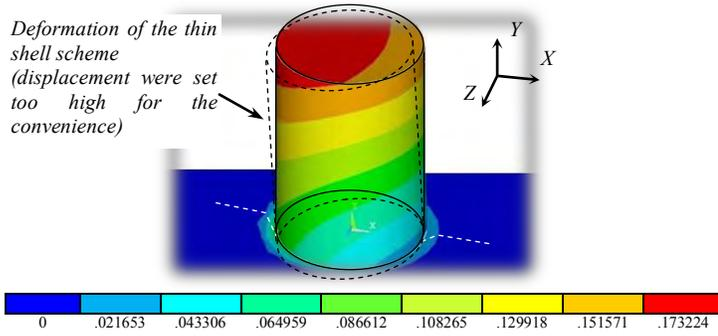
Fig. 7. Total displacement (in m)
