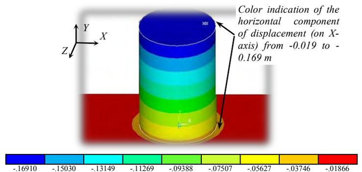
Fig. 6. Horizontal displacements (in m)
