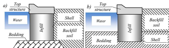
Fig. 1. Layout of a berth made of large-diameter shell: a) the shell on the "rock bedding"; and b) the shell restrained into the existing bedding
