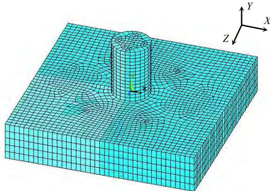
Fig. 3. Finite-element model of a shell with the infill
