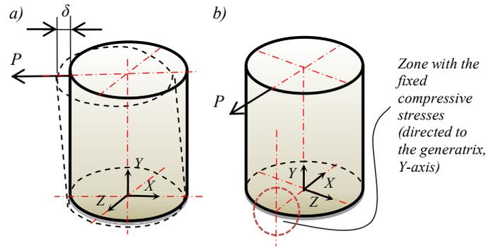
Fig. 12. The fixing parameters a) displacement of the shell top; b) zone with the compressive stresses fixed by strain gauges
