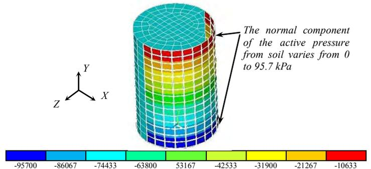
Fig. 4. Soil pressures acting on the shell (in Pa)
