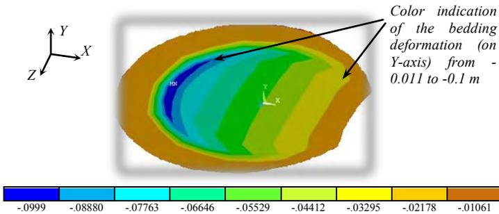
Fig. 8. Bedding deformation (in m)
