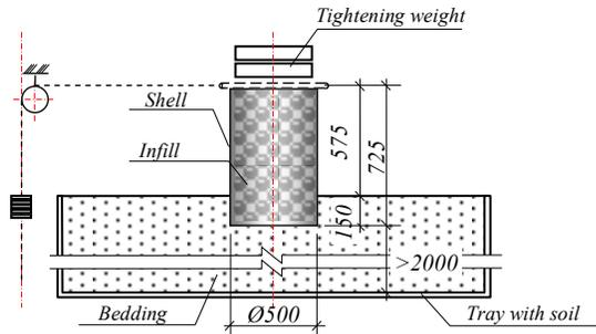
Fig. 10. The schematic and dimensions of the experimental setup device (all dimensions are in millimeters)
