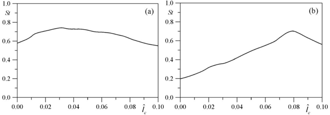
Fig. 4. Impact of single wavefront corrector position on phase aberration compensation efficiency for ten phase screens equally spaced over the distance  $\hat{l} = 0.05$  : (a), (b) ensemble-averaged Strehl ratio versus the normalized wavefront corrector distance for high-resolution phase-conjugated control algorithms for the receiver telescope with infinite aperture (a), and for the telescope aperture coincided with the corrector aperture of size  $D_c$  and  $D_c = 2/3a_0$  (b).
