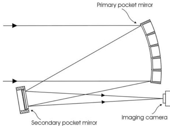
Fig.8. Telescope utilizing pocket mirrors.
