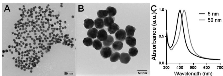
**Figure 4: Characterization of AgNP stock solutions.** Representative TEM images of the experimental (A) 5 nm and (B) 50 nm PVP-coated AgNPs. The images verify spherical morphology and even particle size distribution. (C) The spectral images for both sets of AgNPs in water demonstrate a sharp, single peak.
