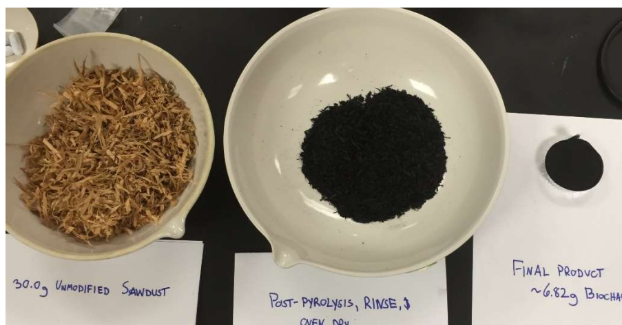
Figure 4.6a: Sawdust before pyrolysis, after pyrolysis, and after final production steps
