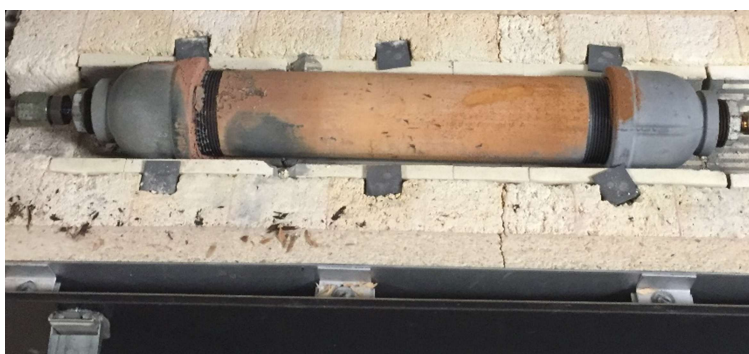
Figure 4.5: Steel reactor for pyrolysis trials
