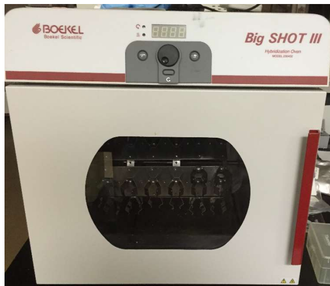
Figure 4.8: Big SHOT hybridization oven used for adsorption isotherm experiments
