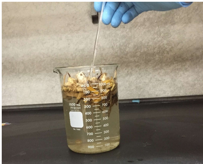
Figure 4.3: Cornstalk acid rinse with manual agitation
