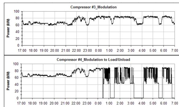
Figure 2. Comparison of compressor power draw between modulation control and load/unload with auto shut-off.
