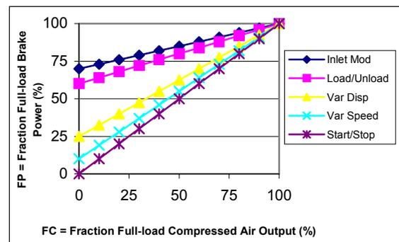
Figure 1. Fraction of full-load power versus fraction of full-load compressed air output for typical reciprocating and rotary air compressors based on type of control.
