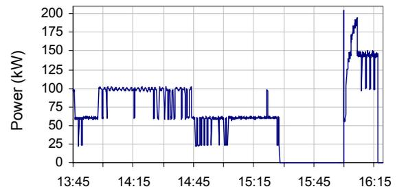
Figure 3. Compressor power draw during plant shutdown showing leak load.
