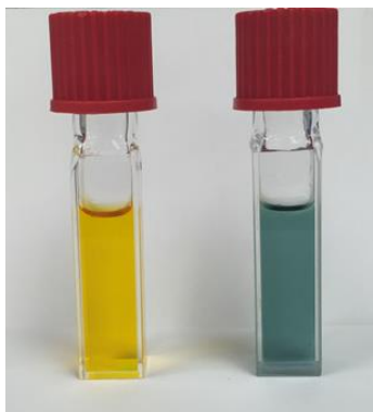
Figure 2. (Left) A 10^{-5}\text{M} solution of \beta -carotene ( \beta\text{C} ) in its native orange-450 state in benzene solvent; (right) A solution of the blue-900 \beta\text{C} -TFA complex in benzene solvent, with [\beta\text{C}] = 10^{-5}\text{M} and [\text{TFA}] = 0.5\text{M} (TFA = trifluoroacetic acid).
