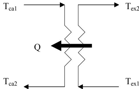
Figure 3. Recuperator schematic
