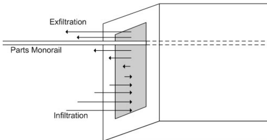
Figure 4. Air velocity profile through vertical oven opening
