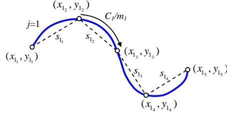
Figure 2: Design profile (solid) with an approximating target profile (dashed) where points are positioned to give a constant arc length along the design profile.
