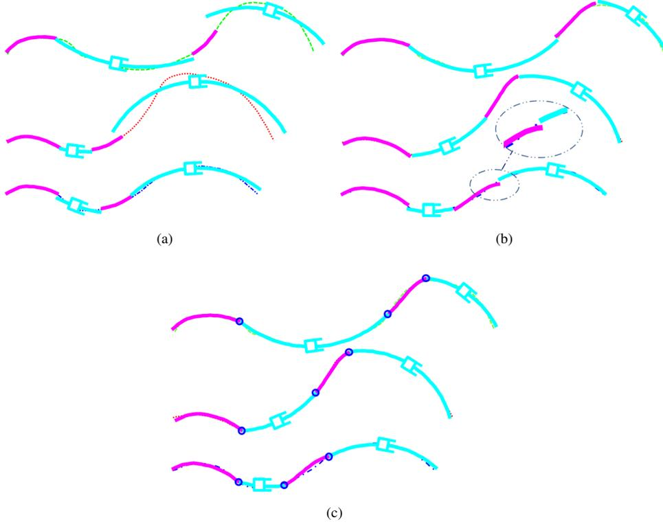
Figure 8: A rigid-body chain that approximates the target profiles. The chain after the initial segmentation matrix is shown in (a) with  $E_{max} = 1.50$ . The chain after the error-reducing iterations is shown (b) with  $E_{max} = 0.33$ . The inset illustrates that segmentation points are not coincident. In (c) the joining process unites segmentation points, yet increases the error to  $E_{max} = 0.34$ .
