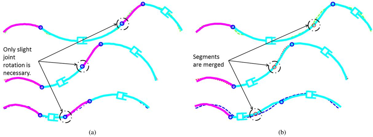
Figure 10: (a) The original chain consisted of 4 segments resulting in  $E_{max} = 0.34$ , yet one revolute joint exhibited limited motion. (b) The 2<sup>nd</sup> and 3<sup>rd</sup> segments were merged into a compound segment, resulting in a three-segment chain with  $E_{max} = 0.46$ .
