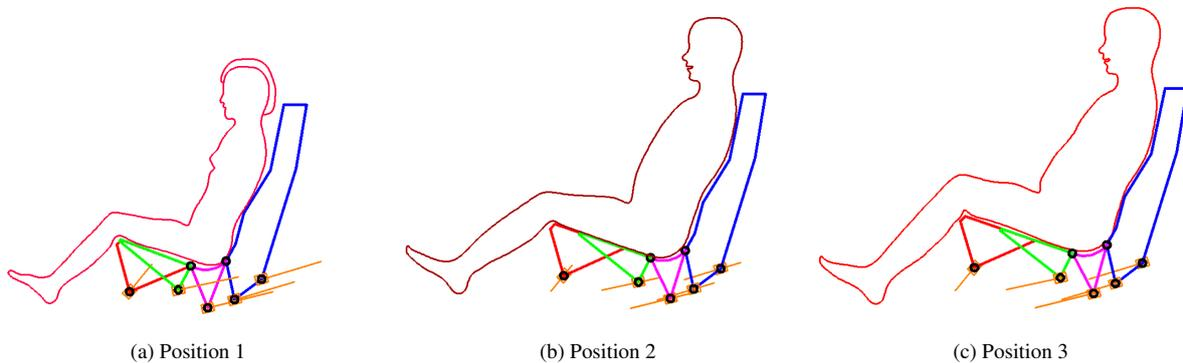
Figure 14: The results of the mechanization process: (a) The seat is adjusted for the small woman. (b) The seat accommodating the medium man. (c) The car seat is positioned for the large person.
