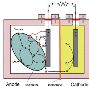
Figure 2: Electron Mediators bringing electrons to the anode (taken from Logan, 2006)
