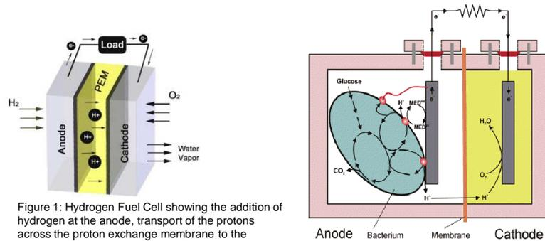
Figure 1: Hydrogen Fuel Cell showing the addition of hydrogen at the anode, transport of the protons across the proton exchange membrane to the cathode where water is generated from  $H^+$  and  $O_2$ . [www.ultracellpower.com/sp.php?fuel](http://www.ultracellpower.com/sp.php?fuel)
