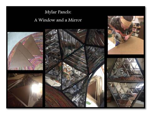
Mylar is flimsy, so it needed a frame around it to keep its structure. I built frames for the mylar using bamboo slats. These slats came in the form of a bamboo fence which I deconstructed and cut to the appropriate lengths. After assembling and gluing these frames I tied the ends with string and used double sided tape to attach them to the mylar.
