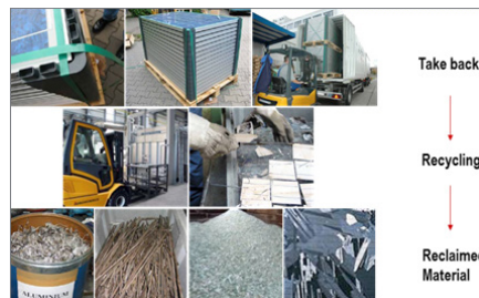
Figure 1-b. Simplified c-Si recycling process and the reclaimed material
