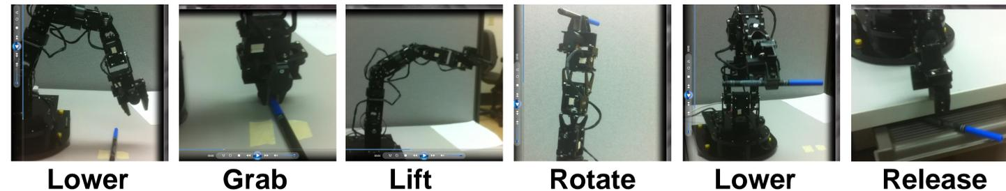
Currently the system maps specific thought patterns through the algorithms provided in the Emotiv SDK shipped with the EPOC headset. Positive classifications are mapped to 6 actions (lower, grab, lift, rotate left, rotate right, and release). Users have been able to execute from one to six of these controls with varying degrees of reliability.
