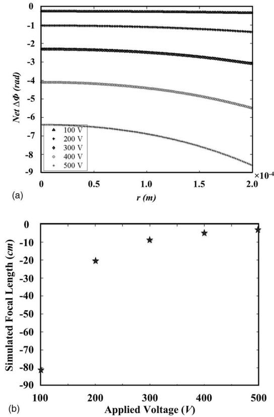
**Fig. 5** (a) The induced net phase change as calculated using COMSOL Multiphysics simulation results, and (b) the corresponding induced focal length variation as a function of the applied voltage. Notice that the induced focal length is negative, and hence we obtain a diverging lens, and that the net phase change increases with higher voltage values, and hence a shorter focal length is obtained. The preceding results are for the x polarization.
