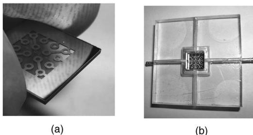
**Fig. 10** The fabrication results of the PLZT microlens array module: (a) 1-cm<sup>2</sup> die, and (b) the packaged lenslet array module.
