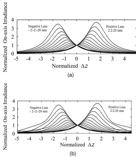
**Fig. 7** Z-scan for linear lenses with focal length values that vary between  $\pm 2$  to 20 mm in 2-mm increments: (a) without aperture diffraction, and (b) with aperture diffraction. Note that the maxima locations are independent of the diffraction effects. Furthermore, the diffraction affects the normalized irradiance amplitude toward the leading edge and the trailing edge of the positive and negative lenses, respectively.
