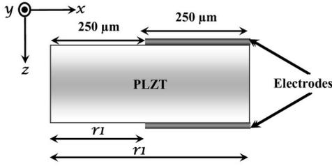
**Fig. 3** Cross-sectional slice of the PLZT microlens structure under test. Note that the cross section is along the  $x$ - $z$  direction and represents one-half of the lens structure. If we revolve this cross section around the  $z$  axis, we will obtain a cylinder where the lens aperture is in the middle, with inner and outer radii of  $r_1$ ,  $r_2$ .
