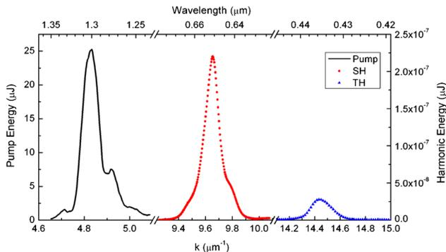
FIG. 5 (color online). Measured spectra of the pump and the transmitted harmonics. The area under each spectrum corresponds to the measured energy ( $2.9 \mu\text{J}$  for pump,  $3.7 \times 10^{-8} \mu\text{J}$  for SH, and  $7.3 \times 10^{-9} \mu\text{J}$  for TH).
