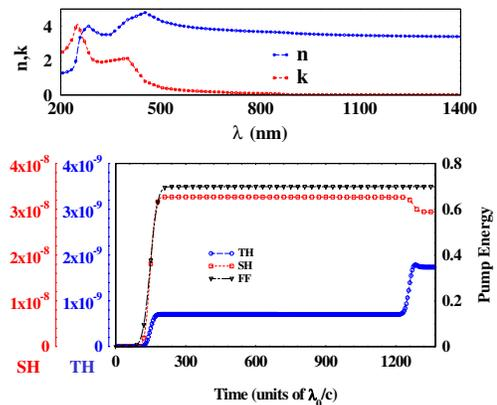
FIG. 3 (color online). Bottom: Pump (right axis) and harmonic (left axes) energies inside and to the right of the substrate. Harmonic generation occurs at entry (time  $\sim 150$ ) and exit (time  $\sim 1200$ ) surfaces, and the energies remain constant inside the substrate. At the exit surface, some SH energy is lost, while the TH signal nearly doubles in magnitude, although opposite behavior is also possible [15] using slightly different material dispersion.
