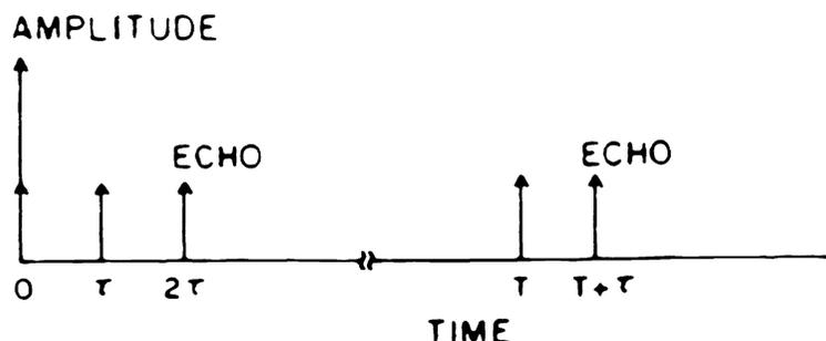
Fig.2.1 Typical sequence for a two- and three-pulse echo.
