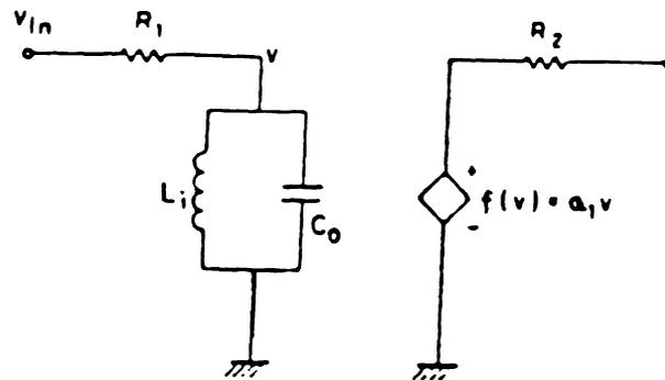
Fig.3.2 Typical circuit configuration used for generating memory echo.
