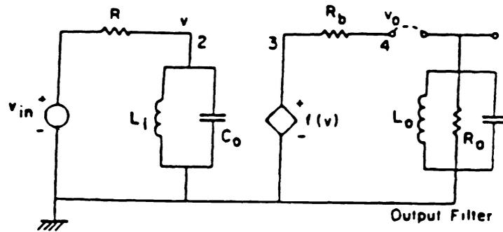
Fig.3.1 Typical nonlinear output coupling configuration.
