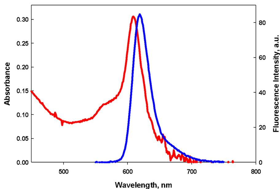
To determine the molar extinction coefficient for BDP 2 at 609 nm, absorption spectra were measured for different concentrations and analyzed using Beer's Law in figures 7 and 8 shown below. Based on figure 8, the molar extinction coefficient was found to be  $80,000 \text{ M}^{-1}\text{cm}^{-1}$ .
