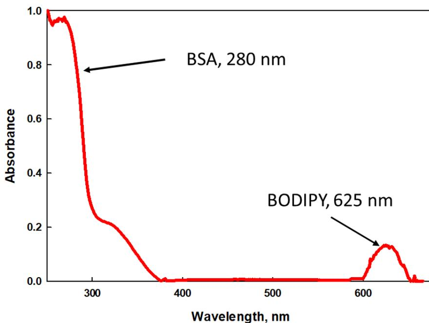
BSA has an intense absorption at 280 nm with a molar extinction coefficient of 44,000  $M^{-1}cm^{-1}$ . BDP 2 has an intense absorption at 625 nm with a molar extinction coefficient of 80,000  $M^{-1}cm^{-1}$ . Analysis of the absorption spectra indicates that only 50% of the BSA protein molecules were tagged with BDP 2.
