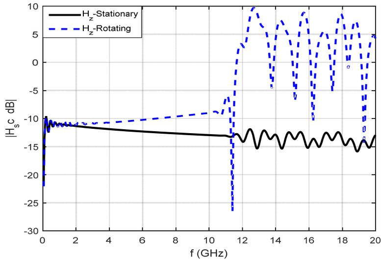
Fig. 6 Magnitude of the backscattered magnetic field as a function of frequency for a very good conducting cylinder, immersed in an incident H-wave ( $\sigma = 5.76 \times 10^7$  s/m,  $a = 0.2$  m,  $\beta_a = 0.0009$ ).
