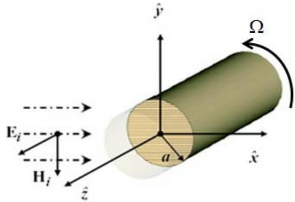
Fig. 1 Rotating conducting cylinder illuminated by E-wave.
