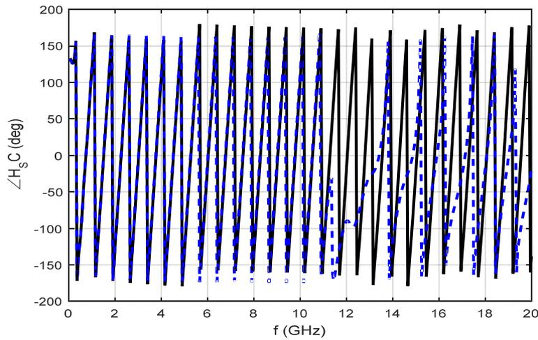
**Fig. 7** Phase of the backscattered magnetic field as a function of frequency for a very good conducting cylinder, immersed in an incident H-wave ( $\sigma = 5.76 \times 10^7$  s/m,  $a = 0.2$  m,  $\beta_a = 0.009$ ).
