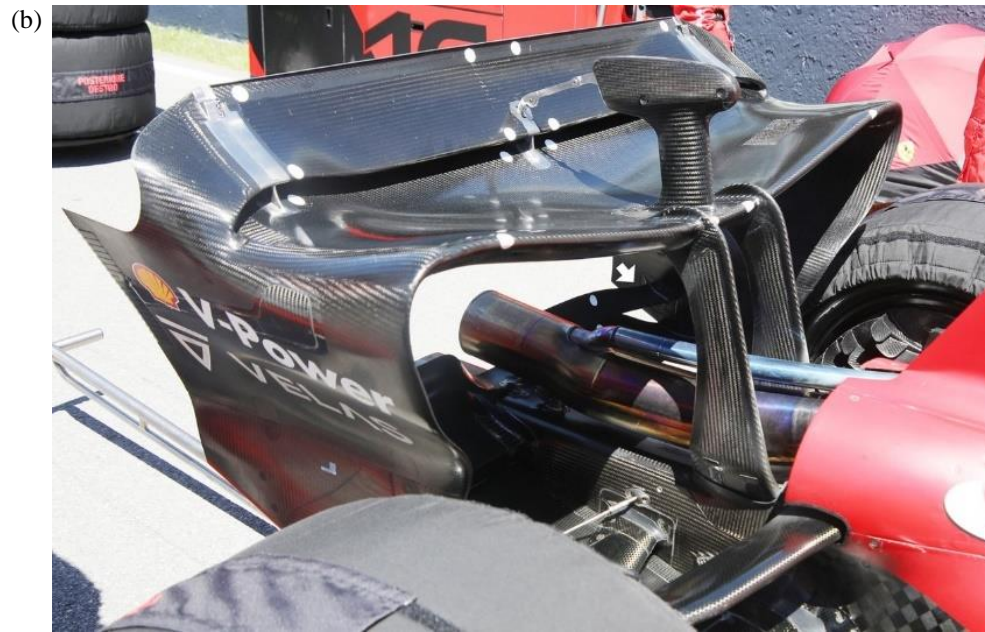
Figure 2: Comparison between the (a) geometric representation of the 2022 F1 rear wing developed in ESP and (b) 2022 F1 rear wing of the Ferrari F1-75. Extracted from Scuderia Fans [11].
