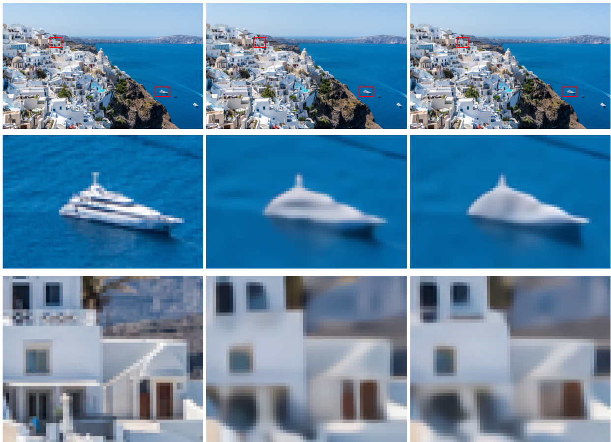
Fig 11 DIV2K Image 823. The truth is shown in the left column, the output of Hex + NI ( 2\times ) + RCAN ( 2\times ) processing is shown in the middle column, and Rect + RCAN ( 4\times ) outputs are shown in the rightmost column. On the first detail row, the hexagonal model captures some notion of a horizontal line corresponding to the decks of the ship, which is absent from the rectangular model. On the second detail row, the hexagonal model renders the brown door better than the rectangular model.
