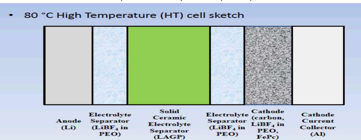
Figure 2: High Temperature (HT) cell sketch.
