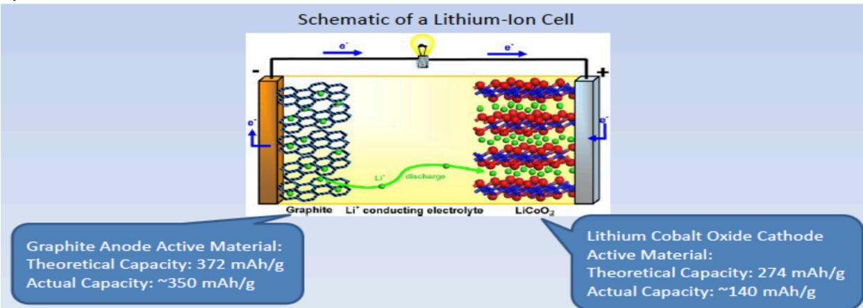
Figure 1: Schematic of a Lithium-ion Cell.
