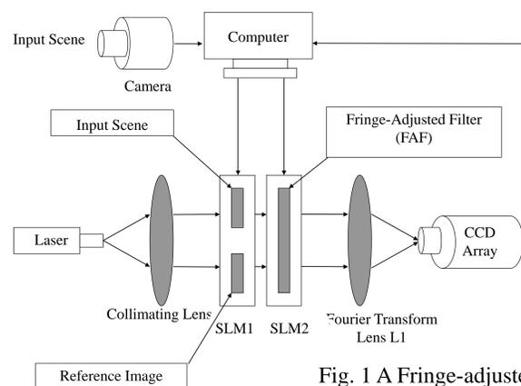
Fig. 1 A Fringe-adjusted JTC architecture.
