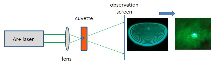
Experimental setup for generating the bubbles. Diffraction patterns for SPM and TB are shown.
