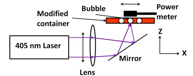
405 nm laser is focused on to the sample and output power is measured in the presence and the absence of bubble
