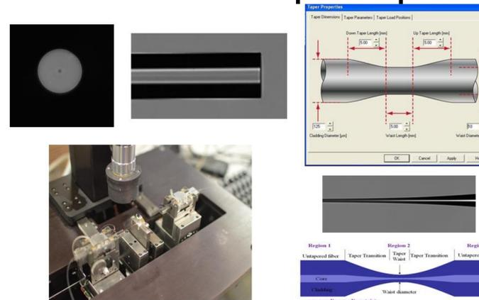
The Vytran GPX-3000 has a high precision for the fabrication of taper device. The system has two holding blocks where each end of the fiber is firmly attached. There is a filament in the center of the system that locally heats the fiber and the entire system is computer controlled
