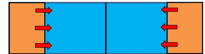
Moving Reaction Front Model: Similar to shrinking core with either a point of symmetry or impermeable material in place of center of a sphere
