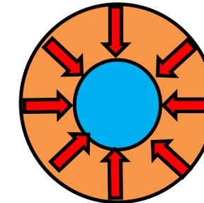
Shrinking Core Model: Reaction occurs at boundary between phases in a sphere
