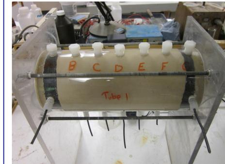
Figure 1. Example of a labelled acrylic tube filled with kaolinite prior to the EKR process.
