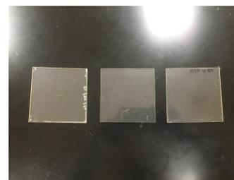
Three resin plaques were successfully produced: no voids or bubbles
