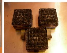
Samples in holder (post test). Smoke and drips came out the bottom on the frame during testing. The final chars from this sample were more sticky than the control chars, suggesting that some of the epoxy was thermally degraded, but not fully decomposed / charred.
