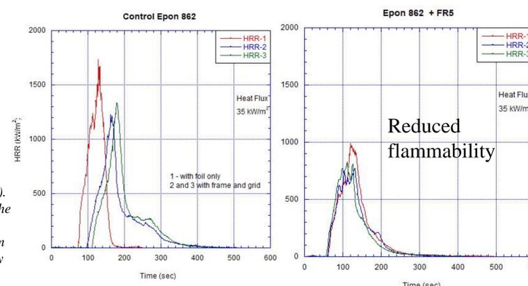
The samples containing FR5 ignited sooner than the control samples but did extinguish a little faster. This indicates the flame retardant helped form a higher level of char which lowered total heat release and resulted in a shorter burning time.
