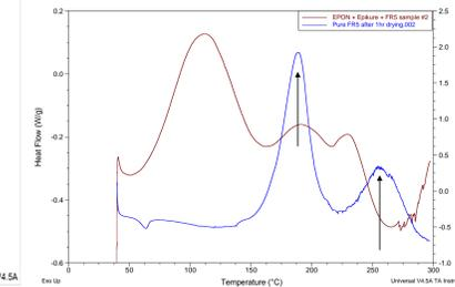
There was a significant difference in the FR5 reaction when cured into the mixture: the 2<sup>nd</sup> exothermic peak shifted to a lower temperature. This may indicate an interaction between FR5 and the network, possibly related to char formation
