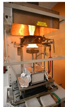
Testing was performed at UDRI with a heat flux of 35 kW/m<sup>2</sup> (acknowledge: Mary Galaska)
