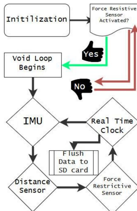
Figure 1: Flow chart of code used to extract data from the cane.
