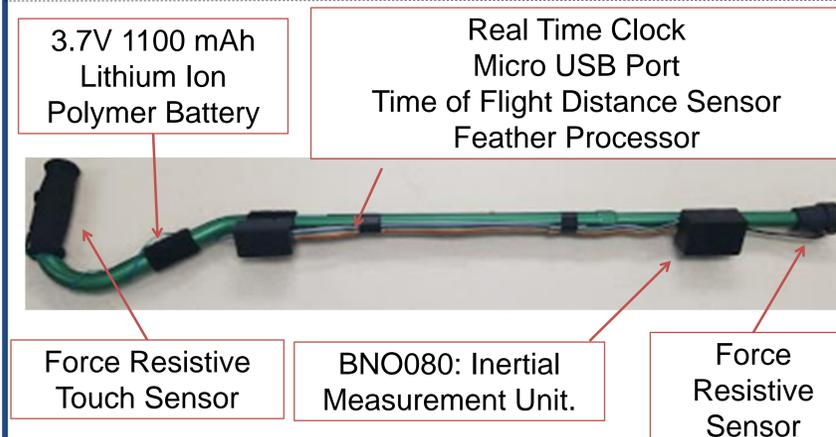
Figure 2: Cane Prototype V.1
