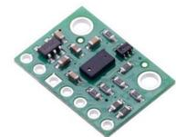
Image 1: VL53LOX Time of Flight Distance Sensor.
