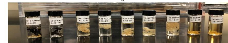
Fig 5: Solubility test of produced nanofibers before and after crosslinking in purified water for 24hrs
