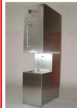
MCC exposes a small sample (5-50 mg) to very fast heating rates to mimic fire type conditions.
