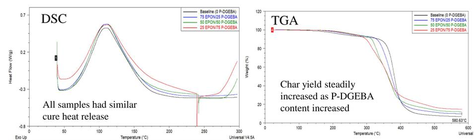
As shown in both DSC and TGA analysis the dilution P-DGEBA by 50% wt. with EPON825 is the best option due to the good balance between both of curing and thermal properties.
