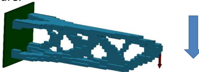
The results are transferred through the interpreter to SolidWorks. An automated routine generates structural tubing members and welds to create a fully manufacturable part.
