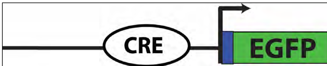
Figure 3. Reporter transgenes include a CRE sequence placed next to a heterologous promoter (arrow) and the coding sequence for an easily monitored reporter protein, such as Enhanced Green Fluorescent Protein (EGFP).
